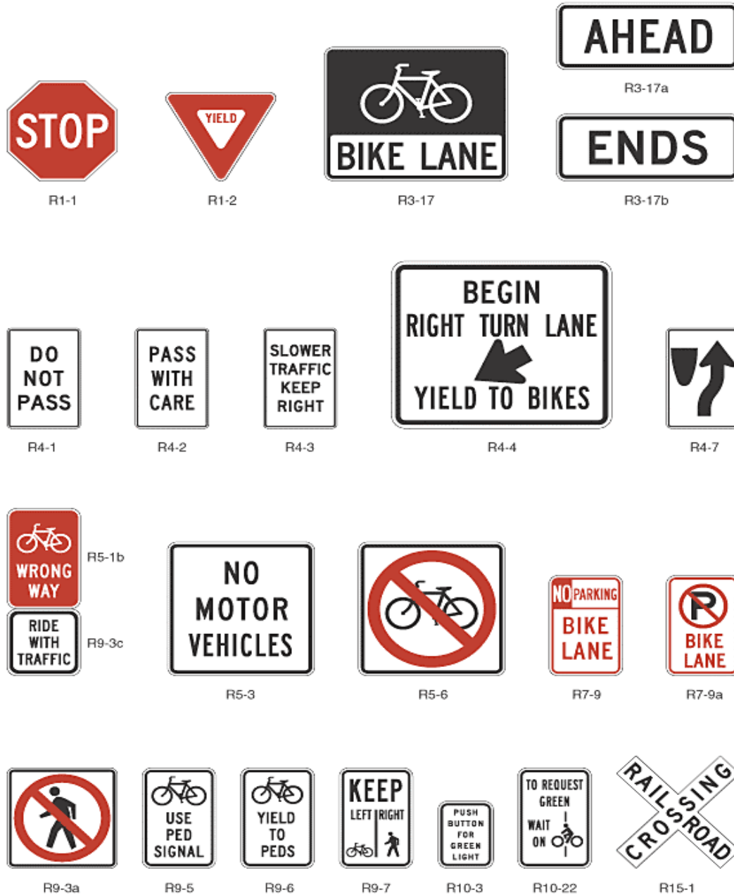
Figure 9B-2. Regulatory Signs for Bicycle Facilities
